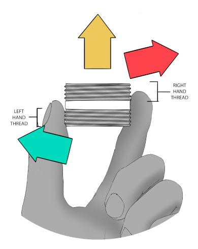
*i* The diagram to the left shows how to recognise the two thread directions of a double threaded nipple used to join cast iron radiators.
