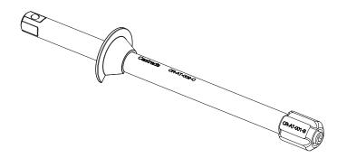
If the nipple doesn't screw in easily it's likely that it has been inserted the wrong way. If this is the case, undo the join and check the thread orientations. It is important not to force the thread as this will damage the radiator and cause a leak.
